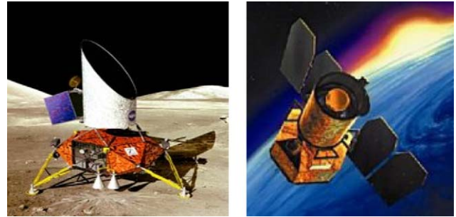
Fig. 1. Artist's rendering of (left) the Lunar Ultraviolet Telescope Experiment (LUTE) concept ca 1993, and (right) the Galaxy Evolution Explorer (GALEX). GALEX was successfully launched in April 2003 as part of the NASA Small Explorer (SMEX) program. Both were designed to operate autonomously as ultraviolet survey telescopes, offering similar light collecting aperture and spatial resolution, roughly comparable deployed mass and power budget, with design lifetimes of two years. LUTE was conceived as a small-field transit instrument operating on the lunar surface, while GALEX is an all-sky survey mission in LEO. At the time that GALEX was competitively selected by peer review, the SMEX program had a cost cap of $120M per mission including development, launch, mission operations, and data analysis. Now successfully implemented, GALEX has been a highly economical approach to ultraviolet survey astronomy.
